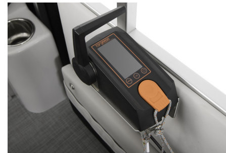
Torqeedo Cruise 2.0 24V System, Comparable to a 6 HP gas engine. Battery information center in throttle with GPS.
