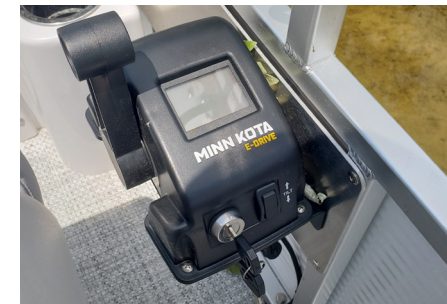
Minn Kota E-Drive 48V System, Comparable to a 5 HP gas engine. Integrated power tilt & backlit battery gauge in throttle.
